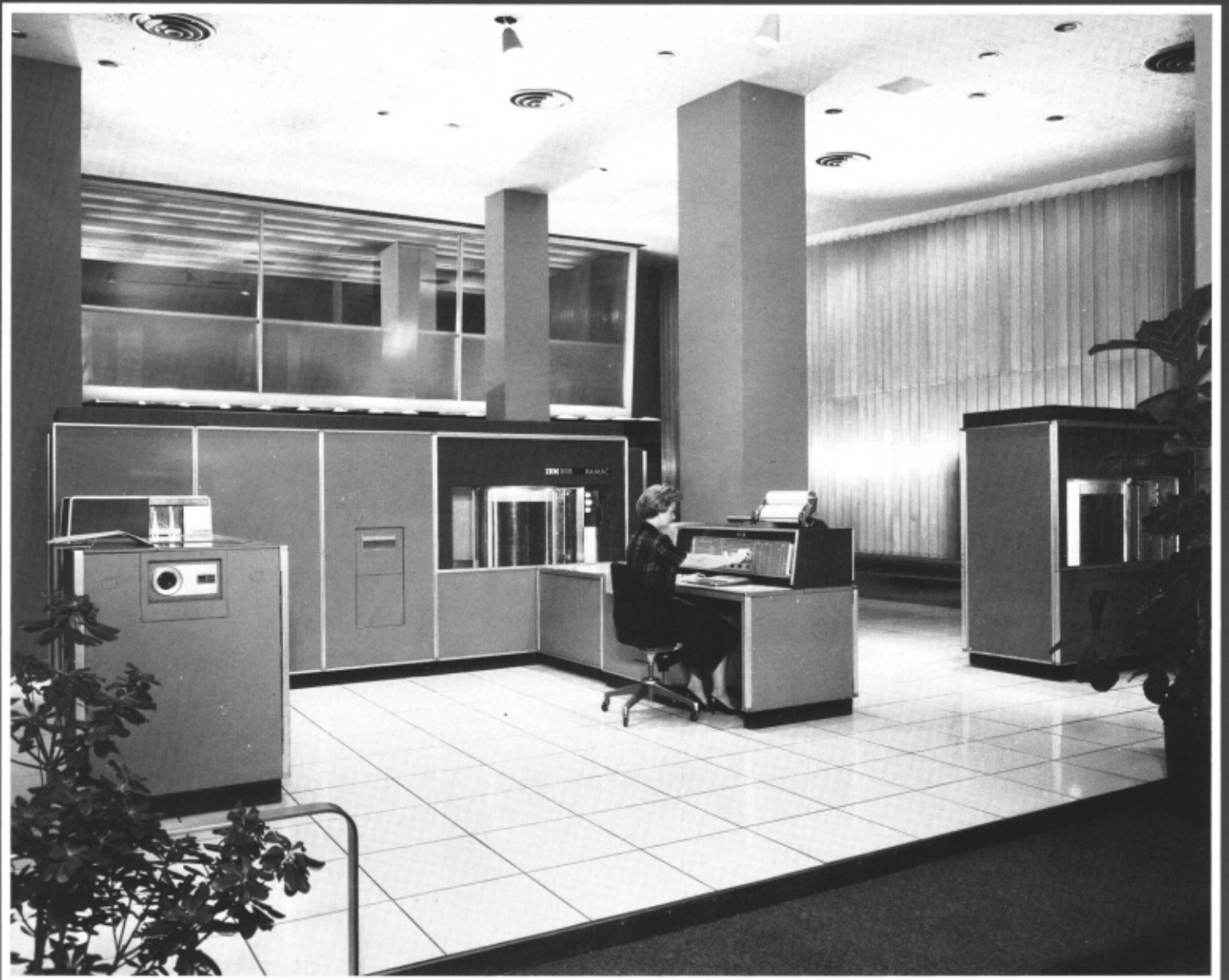
One of the press release photos for the 305 RAMAC System when it was first announced in 1956. Key component was the 350 disk file. The system also included a central processor, card reader and printer.
